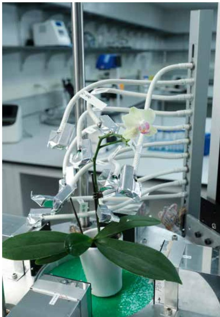
*The BioPETx installed at the Saskatchewan Centre for Cyclotron Science at the Fedoruk Centre. (Photo credit: Fedoruk Centre)*
